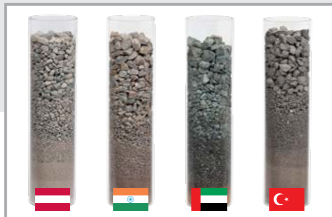
Examples of concrete mixes from 4 countries (from left to right): rounded gravel from Austria, broken stones from India and Dubai, the sample of aggregate from Turkey on the far right was particularly sharp and hard. The grading curves of the aggregate range from fine (bottom) to coarse (top).
