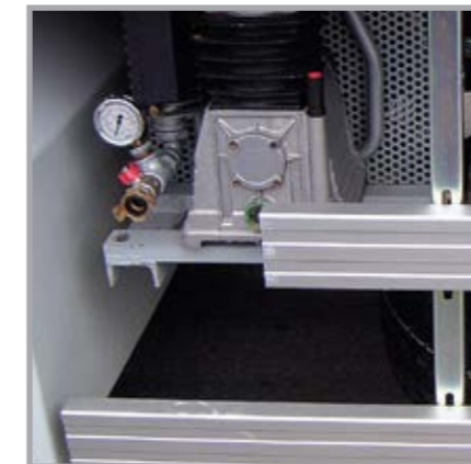
Economical compressor operating at 455 l/min and generating 12 bar pressure – with compact dimensions, mounted behind the lateral underrun ride guard.
