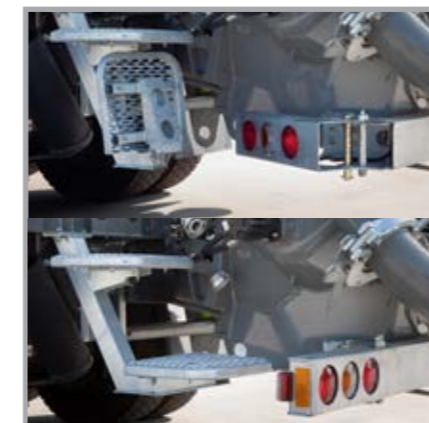
Folding steps in order to prevent damage when filling with two truck mixers.
