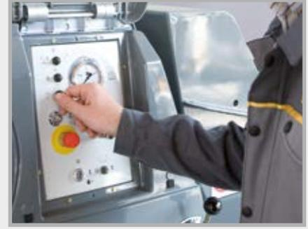
The easy to read, analog instruments and robust switches are protected by a sturdy flap against dirt and the risk of being damaged.
