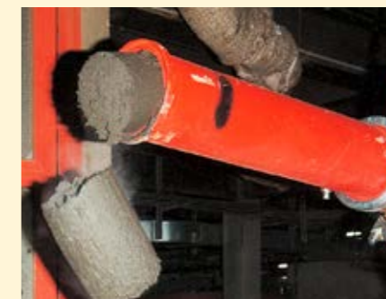
Sewage sludge from filter press and centrifuges
