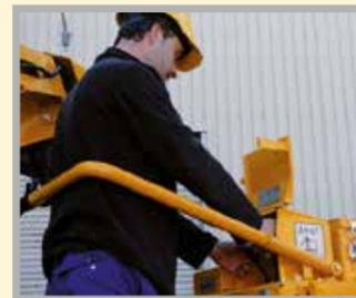
Levers for manual control of crawler in case of emergency
