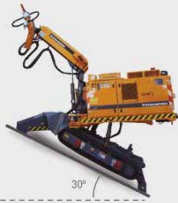
system assures that the correct spraying angle and a stable arm reach are maintained during the spraying process. The hydraulic blade-type stabilizer installed in the rear guarantees the equipment's stability in ascending slopes. In descending slopes, the electronically operated winch with 50 m cable and 6.803 kg traction force is applied.
