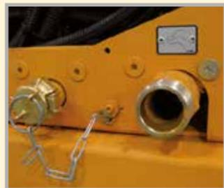
Quick couplings for concrete, additive and air supply. Without disturbing hoses on the sides of the machine
