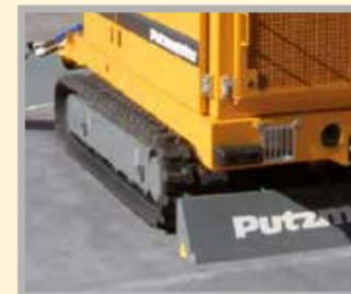
Hydraulically operated rear blade-type stabilizer for safe work in deep ascending slopes
