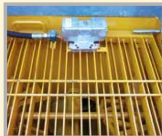
Agitator in hopper and grill with electric vibrator. Steel or polymer fibre pumping. Easy to open for maintenance and cleaning
