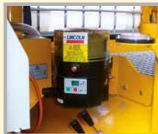
Centralized lubrication system for proper machine maintenance
