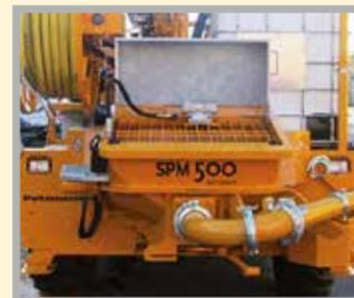
The large diameter and long stoke minimize pulsations and lengthen the life of the concrete pump wear components
