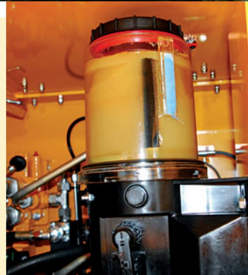
Automatic lubrication system of the concrete pump for proper machine maintenance
