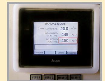
Control system with multilingual colour display, indicating concrete flow, additive dosage, faults, diagnoses and alarms.
