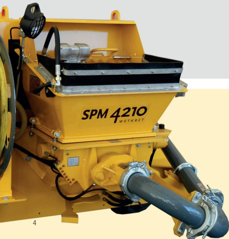
Hopper designed for concrete spraying: Agitator in hopper and grill with adjustable electric vibrator, for steel or polymer fibre pumping. Easy to open for maintenance and cleaning
