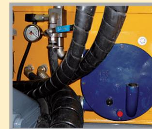
Liquid additive pump, synchronized with the concrete flow.
