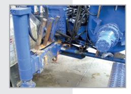
The hopper and agitator are cleaned, the agitator motor is sealed
