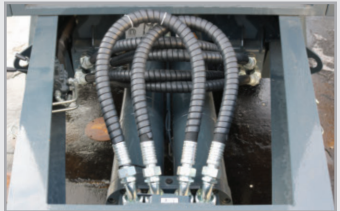
Optional rod/piston change-over system is designed to be fast and easy to facilitate output or pressure, when needed.
