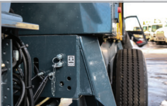
An auxiliary hydraulic connection is included on 2100 and 14000 pumps to operate stand-alone diversion or shutoff valves.
